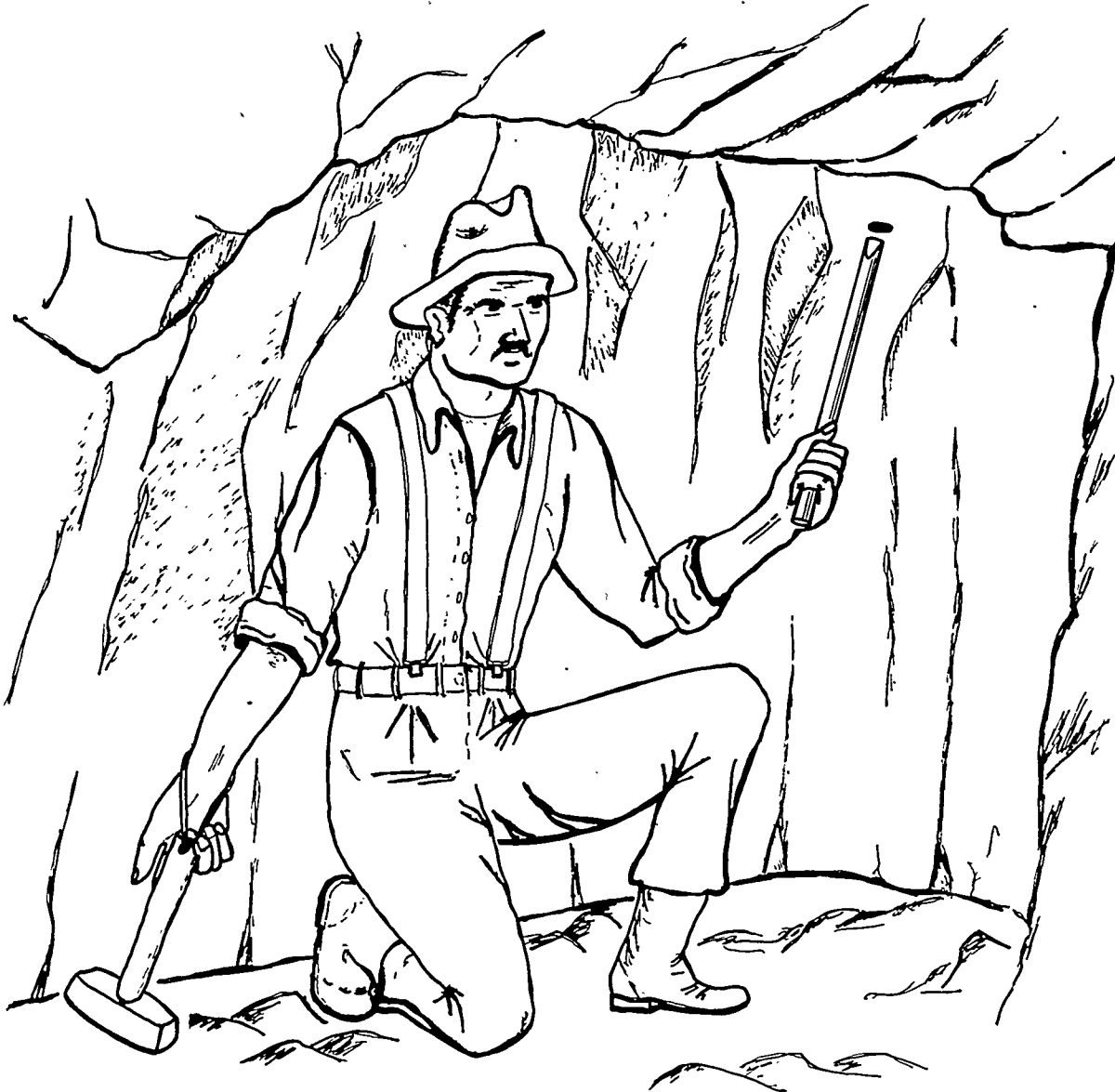
Old time miner using a single jack equipped with wrist thong, early 1800's.
