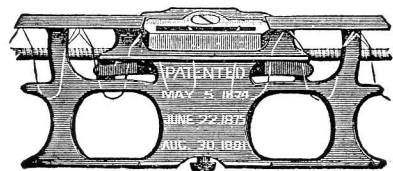
Figure 2—Cutting down rakers Excelsior Raker Gauge
